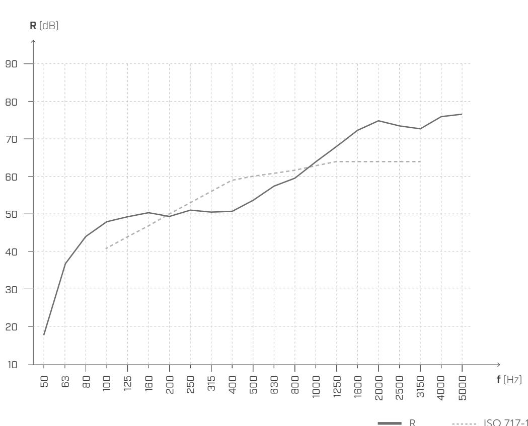
$$R_w(C;C_{tr}) = \text{60} \text{ (-1;-4) dB}$$
